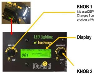
It is as a DEFAULT the CCT Variation Knob, By rotating it clockwise the CCT Changes from 2.750°K up to 6.900 °K. If such a knob is kept pushed, it provides a FAST ACTION on the KNOB 2 which is normally the DIMMING
