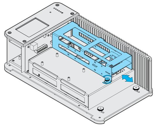
4 Align the Drive Card with the chosen slot and ensure that it engages with the corresponding card guide. Push the card fully into the slot so that the release lever locks into place.
