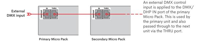
The DMX/DHP ports use RJ45 sockets and can accept standard Catx link cables. The signals are arranged as follows:
