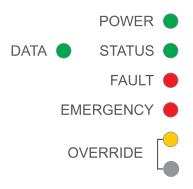
POWER Solid red when the unit is in standby; green when on.
