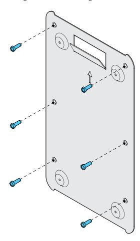
2 Hang the enclosure onto the angled plate of the wall bracket and fix in place using the provided thumb screws.
