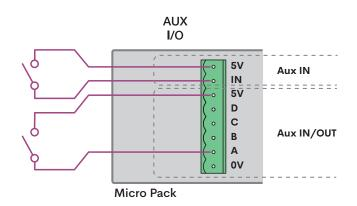
The AUX IN port is a 'dry contact' type and supplies 5VDC on the lower pin. When the 5VDC pin is connected to the IN pin, an ON or logic 1 state is registered and the controller will act upon it, as configured through the menu. When the pins remain open contact, an OFF or logic 0 state is observed.
