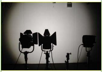
The Beam in full flood is LARGE (above 60°), even and flat (No Hot Spots and rapid passage from Beam to Field Angle)
